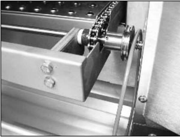
23. Pull the drive coupling back and line it up with the conveyor drive shaft.
